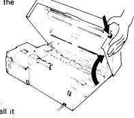
Take out the empty roll and pull out both spools. Insert the spools in a new paper roll and install it with the leading edge at the top of the roll and facing the front of the machine.
